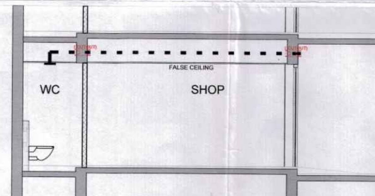
TYPICAL MECHANICAL VENTILATION SECTION
