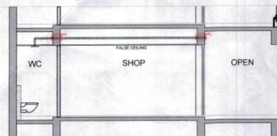
TYPICAL MECHANICAL VENTILATION SECTION
