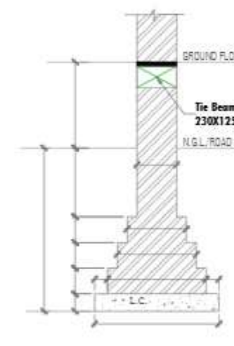
TYP. SECTION FOR 200 THICK BLOCK WALL (Scale: 1:20)
