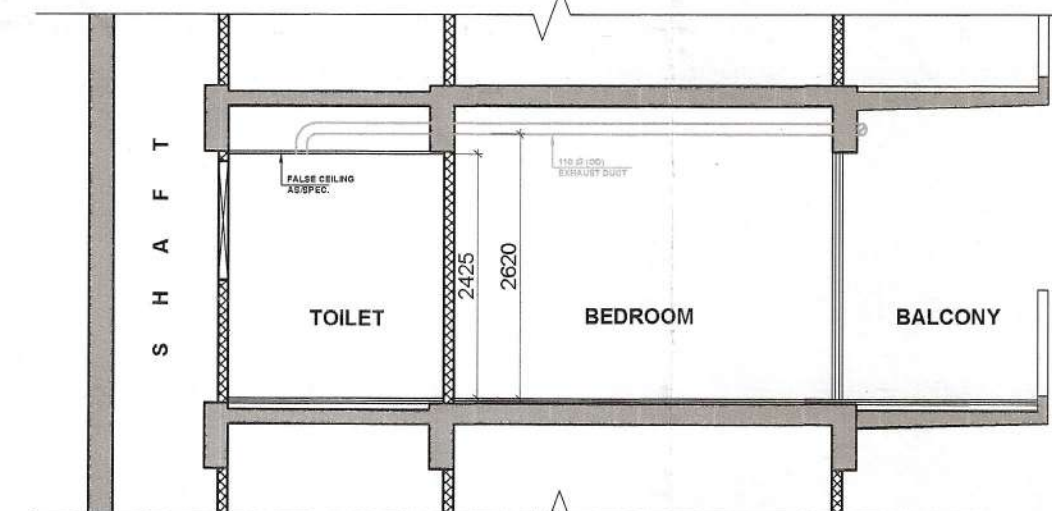
TYPICAL SECTION FOR TOILET VENTILATION
