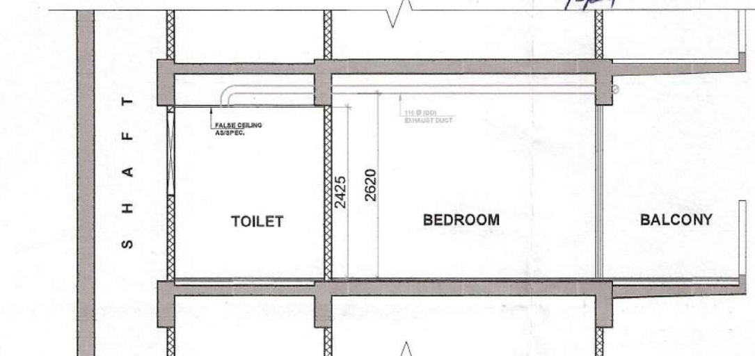
TYPICAL SECTION FOR TOILET VENTILATION
