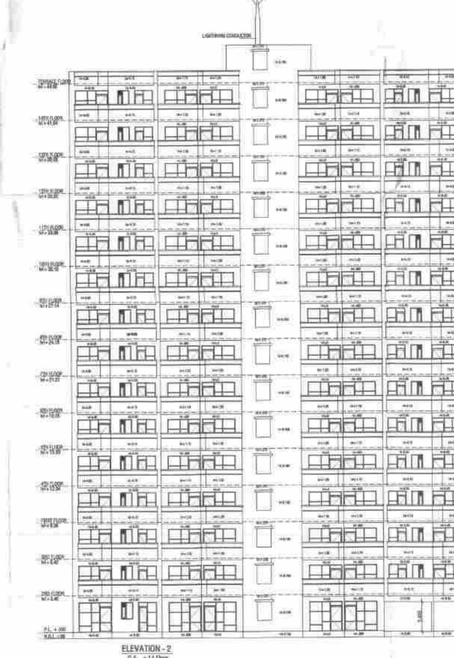
ELEVATION -2 (G.F. to 14th Floor)
