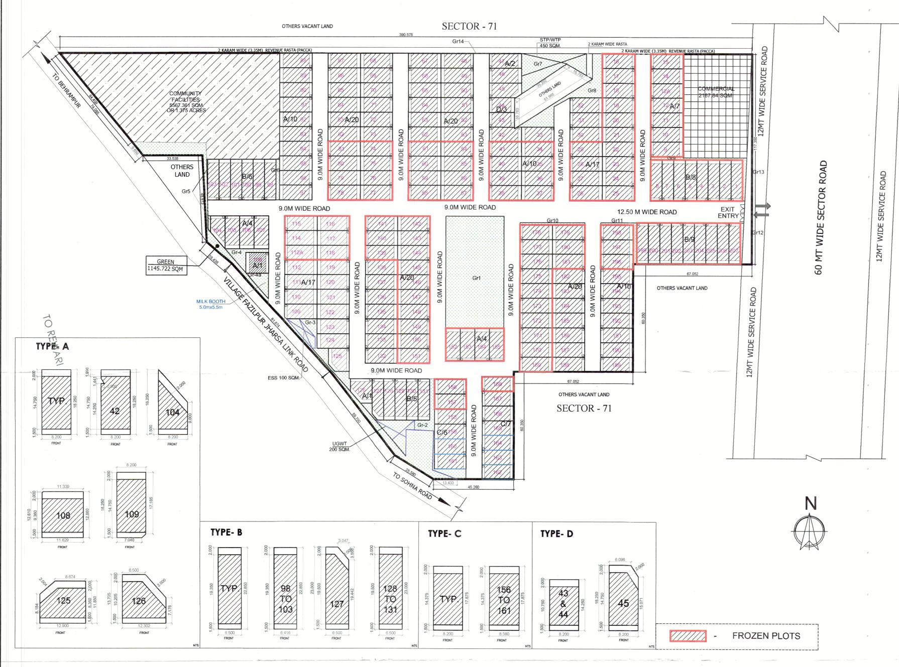
NOTE:- NO PROJECTION/CANTILEVER ALLOWED IN THE REAR SETBACK. ALL DIMENSIONS ARE IN METERS
