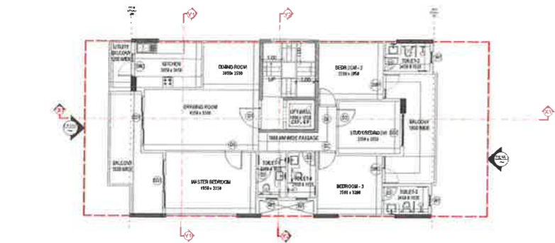
TYPICAL FLOOR PLAN TOILET 1 & 4 ARE MECHANICALLY VENTILATED
