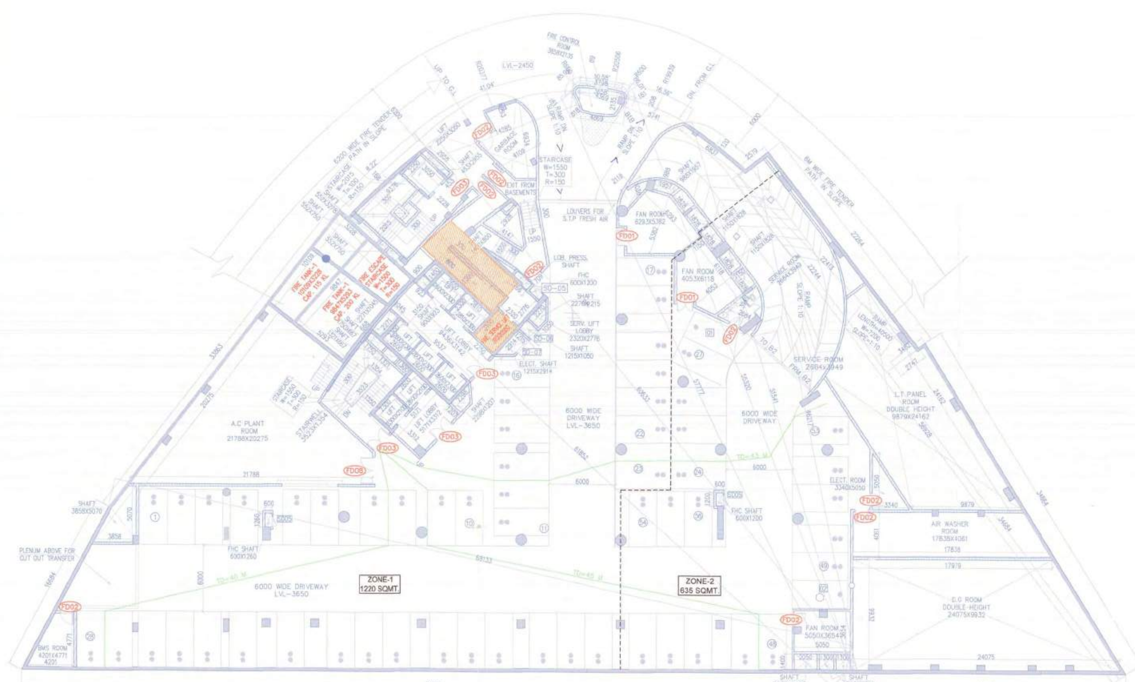
BASEMENT-01 DOUBLE STACK PARKING=56X2 =112 SINGLE PARKING=2 TOTAL NO. OF PARKING = (112+2)=114 Nos. LVL-3650
