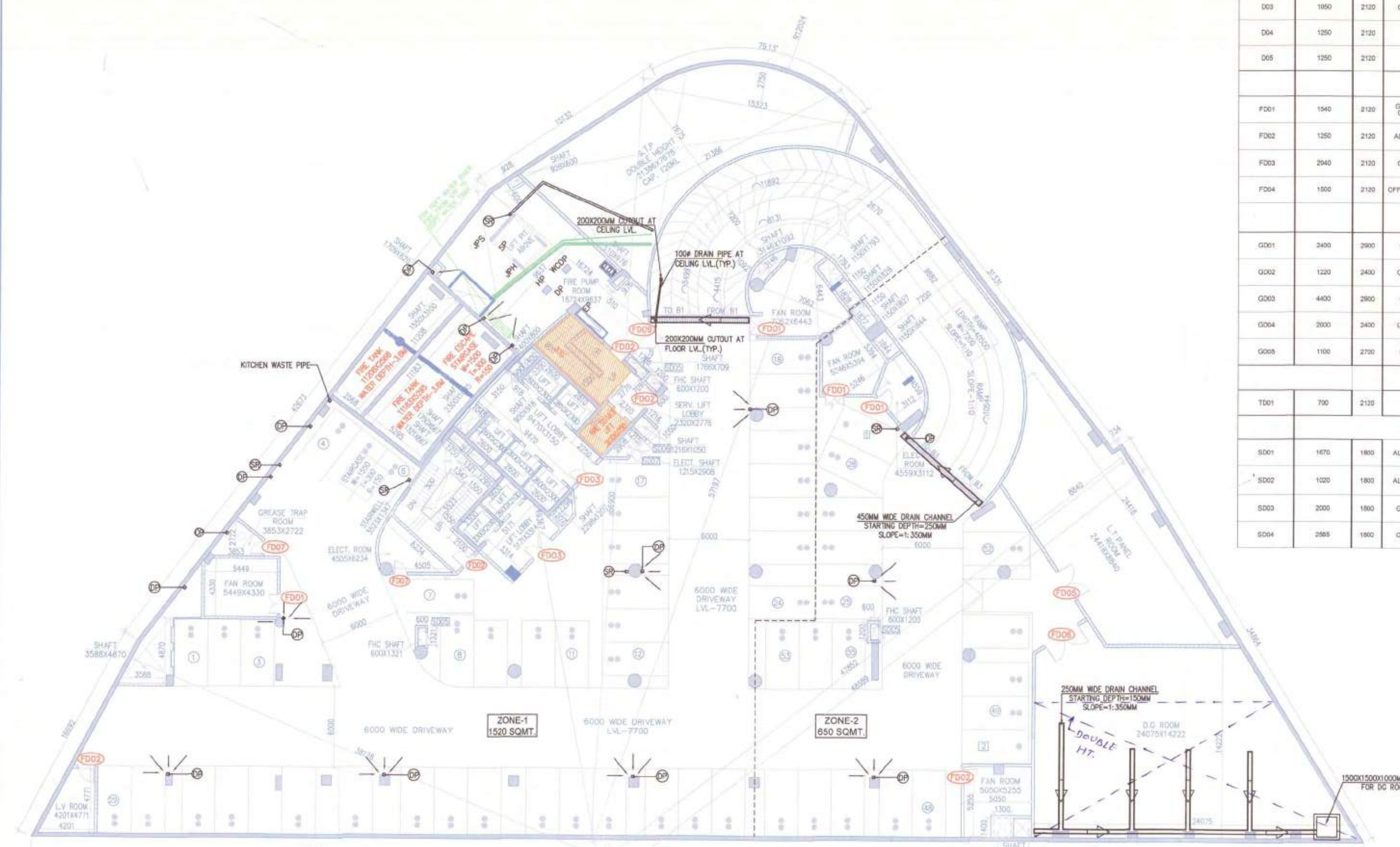
BASEMENT-02 DOUBLE STACK PARKING=55X2 =110 SINGLE PARKING=2 TOTAL NO. OF PARKING = 112 Nos. (110+2) LVL-7700
