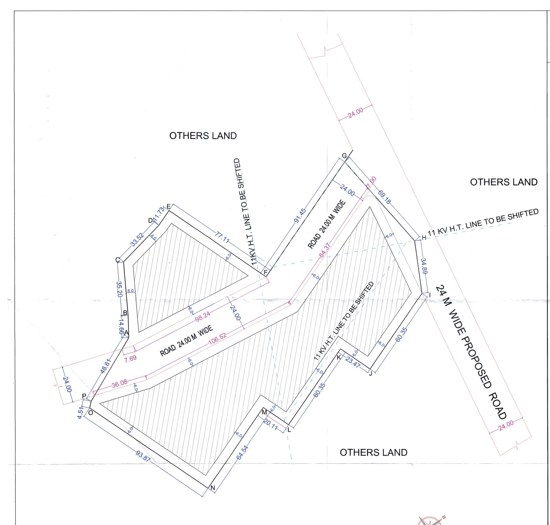
NOTE:-THE APPLICANT SHALL GET 11 KV HT LINES RE-ALIGNED FROM THE SITE BEFORE SUBMISSION OF AMENDED BUILDING PLANS TO BE SUBMITTED IN ACCORDANCE WITH THE REVISED ZONING PLAN OTHERWISE ROW UNDER 11 KV HT LINES SHALL BE PROVIDED IN THE BUILDING PLANS AS PER NORMS.
