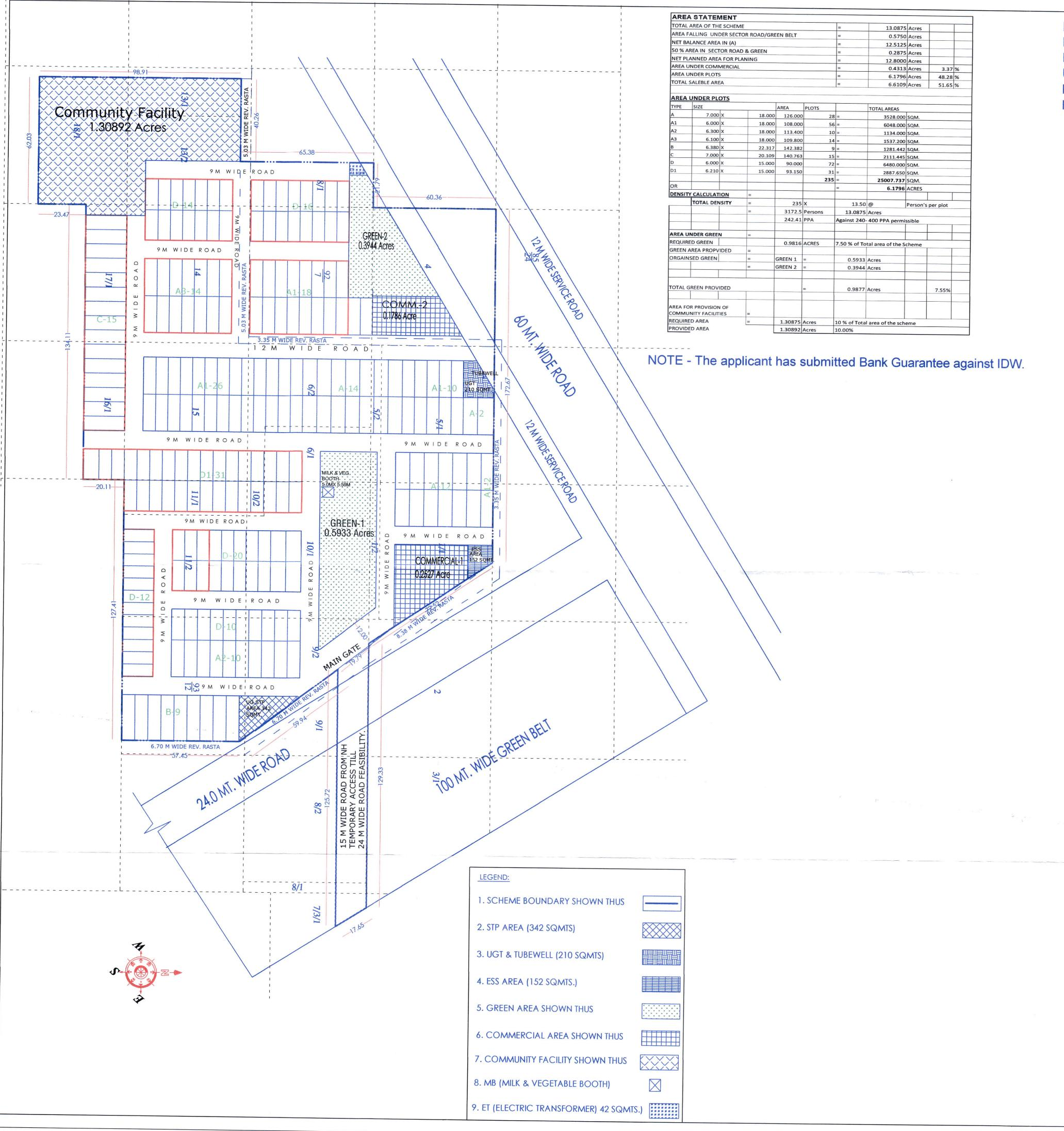
LAYOUT PLAN OF RESIDENTIAL PLOTTED COLONY OVER AN AREA MEASURING 13.0875 ACRES UNDER DDJAY-2016 FALLING IN THE REVENUE ESTATE OF VILLAGE KOT BEHLA, SECTOR -16, KOT BEHLA URBAN COMPLEX , PANCHKULA BEING DEVELOPED BY PIGEON INFRASTRUCTURE LTD. IN COLLABORATION WITH ELDECO INFRASTRUCTURE & PROPERTIES LTD.
