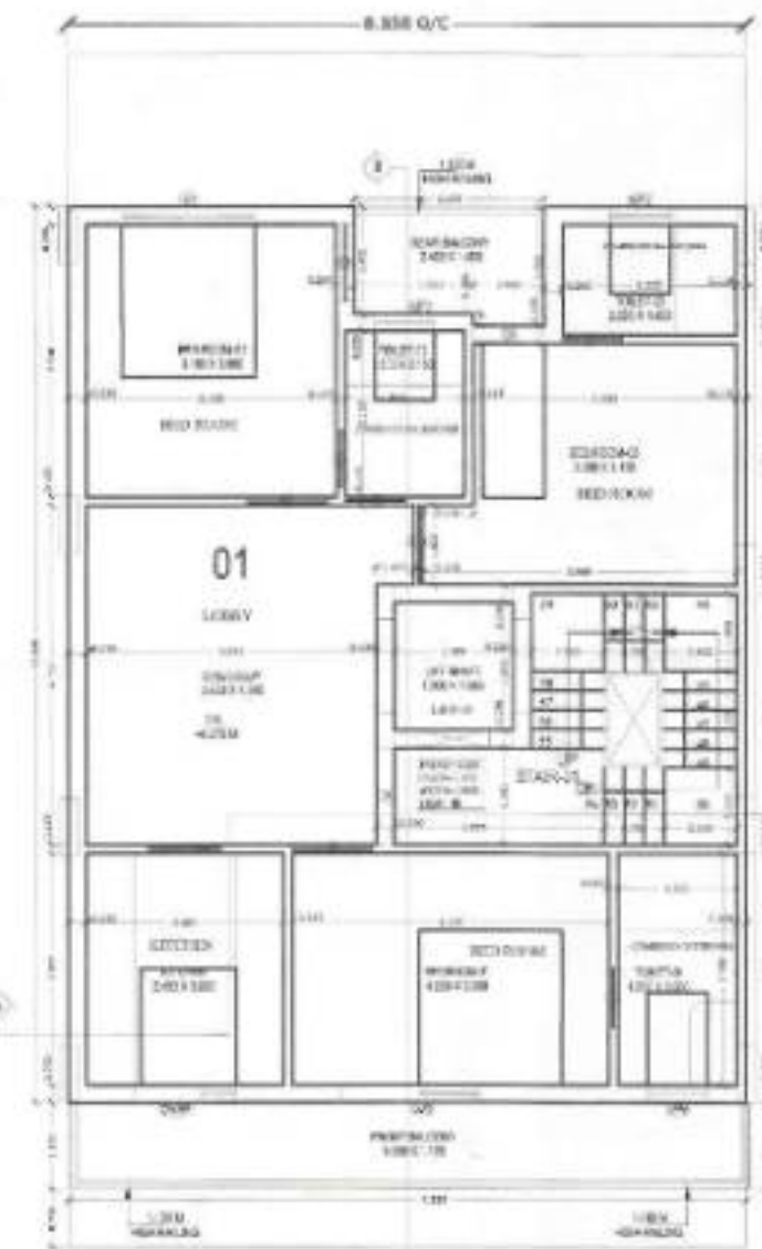
SECOND FLOOR PLAN SCALE 1:50
