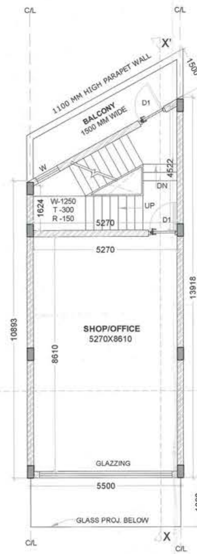
TYPICAL FLOOR PLAN (1ST, 2ND & 3RD)
